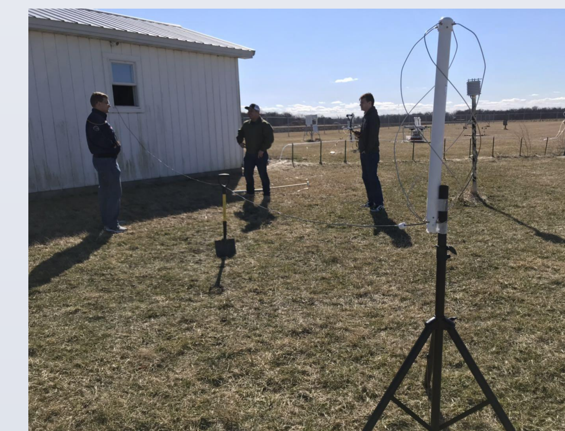
Figure 4: Helix antenna testing (located at Purdue ACRE)
